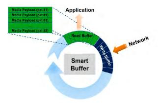
Figure 2: Smart Buffer Management with Mellanox Rivermax
