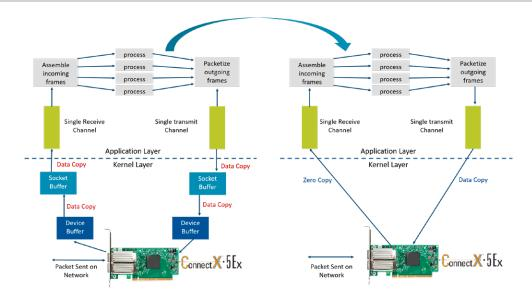
Figure 1: Zero-Copy with Mellanox Rivermax
