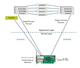
Figure 3: Smart Protocol Offload Enables Kernel Bypass
