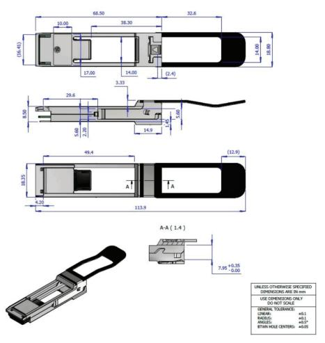
Note: The SFP+/SFP mating paddle card dimension A10 (length of component/solder mask keep-out area, refer to SFF-8071) shall be >6.0mm instead of >5.5mm. The reason for this requirement is to prevent damaging the adapter when trying to insert an SFP upside down.
