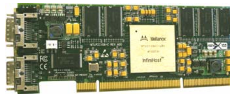
Figure 6. InfiniHost MTLP23108 Low Profile PCI-X HCA Card
