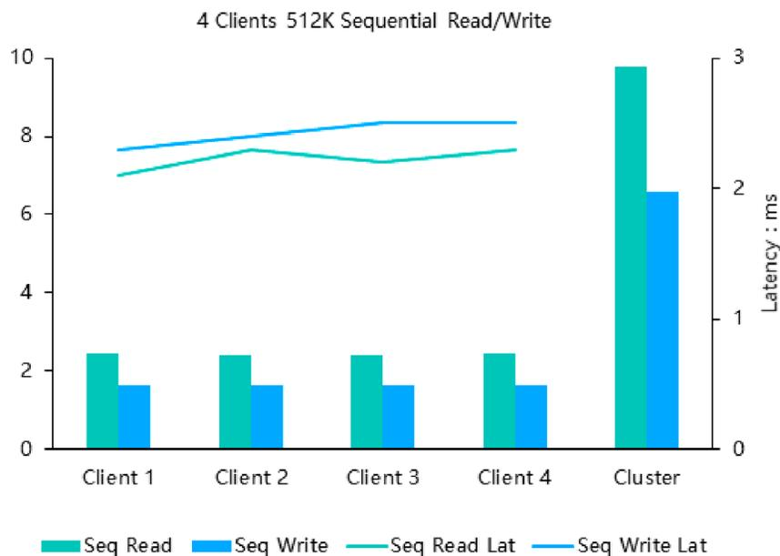
Figure 5: 512 sequential read/write test: 4 clients
