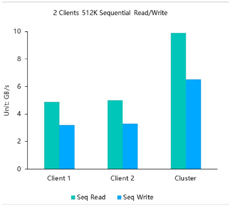
Figure 4: 512 sequential read/write test: 2 clients
