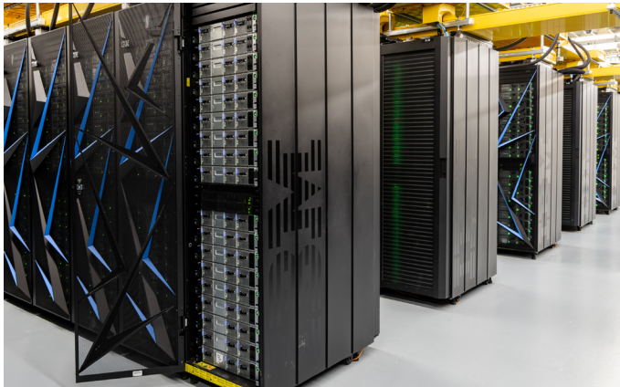
Figure 3: Summit houses more than 10 petabytes of memory with fast, high-bandwidth pathways that allow moving data efficiently.
