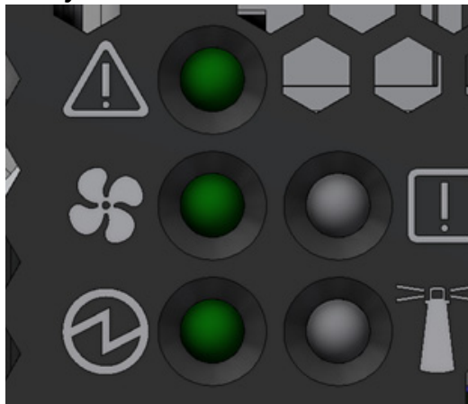
Figure 27: System Status LEDs 5 Minutes After Power On
