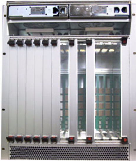
Figure 5. ATCA 3.0 Shelf Prototype (photo courtesy Rittal Corporation)
